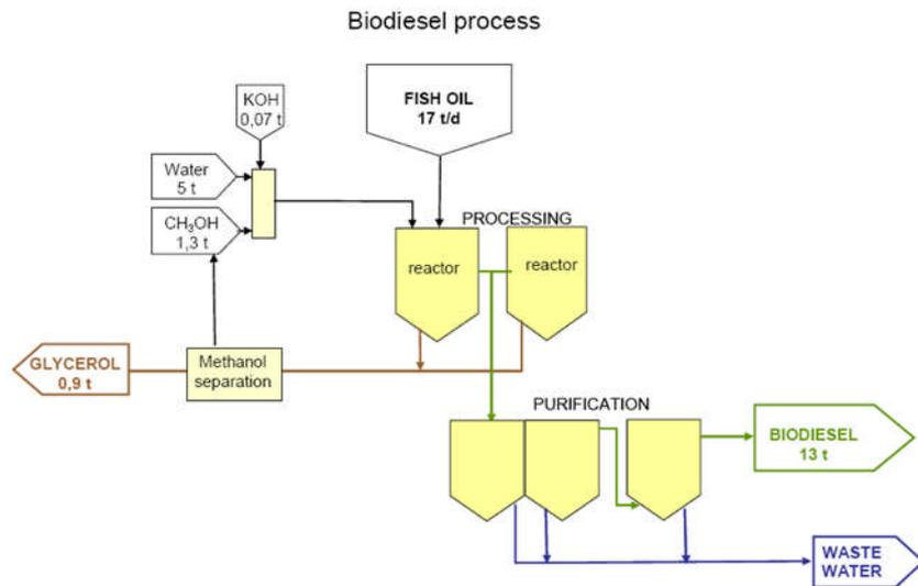
Fig.6 The Preseco Biodiesel PROCESS
