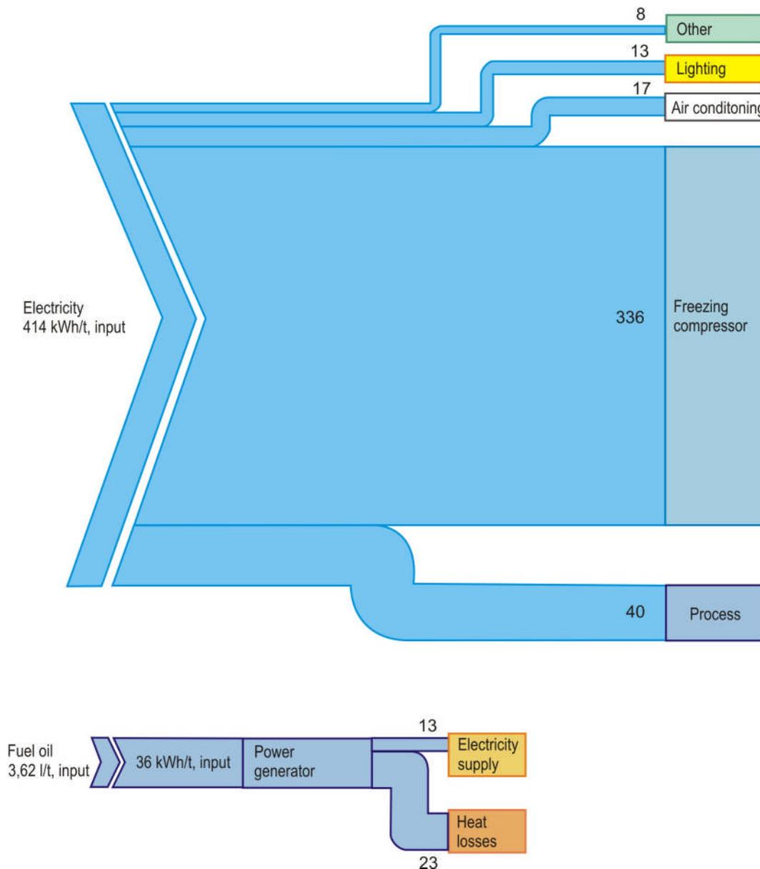
**Figure 3. Energy characteristic use at fish processing factory allocated to the fish intake.**
