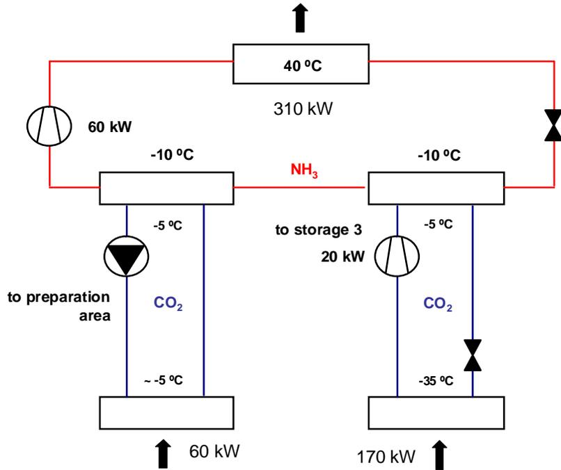
Fig 5 High Efficiency NH<sub>3</sub>/CO<sub>2</sub> Cascade (see Lee et al., Int. J. Refrigeration 29 (2006), 1100)
