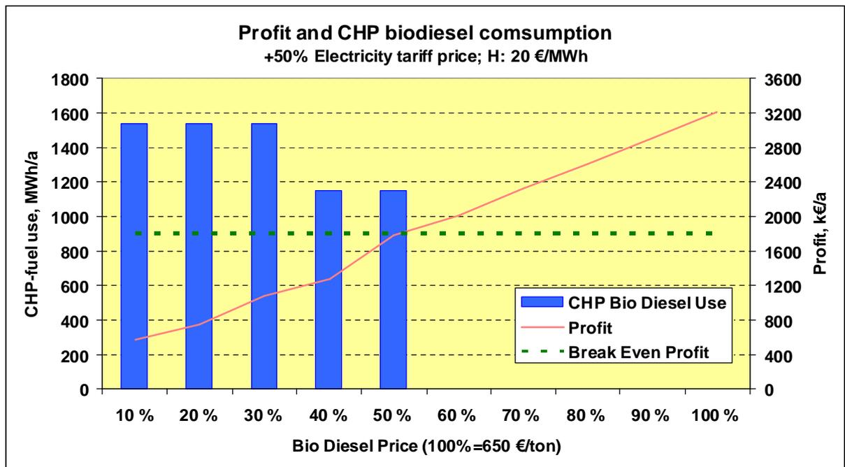
Figure 9. Economical use of cogeneration, and profit of biodiesel fuel alternative as a function of biodiesel market price. Electricity tariff +50 %, price of heat energy is 20 €/MWh.
