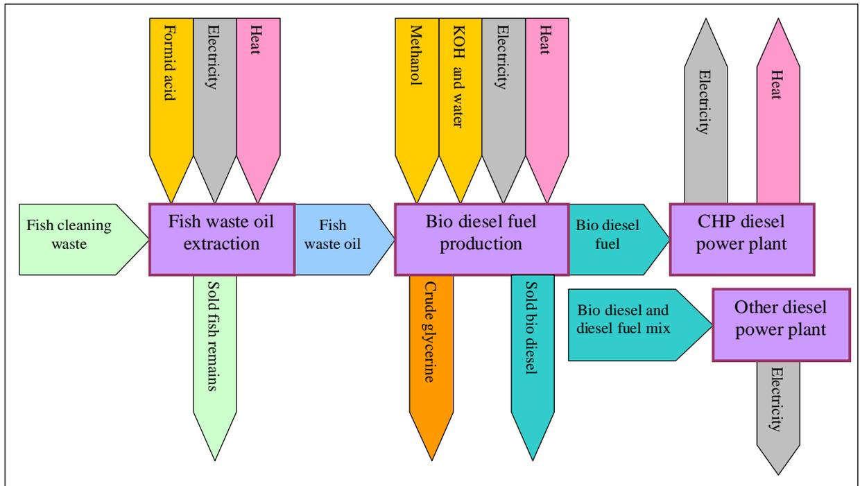
**Figure 7. Process flow chart of the fish oil based bio diesel production used in optimization model.**
