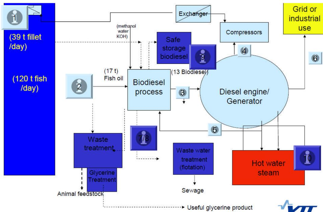
Figure 4. Integration of energy and mass flows at a fish processing factory.
