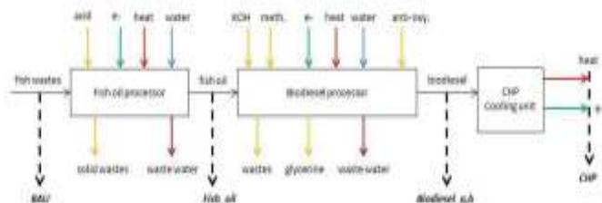
Fig. 1. Schematic view of the Enerfish process. Dotted arrows: business models. Acid: formic acid, e-: electricity, KOH: potassium hydroxide, Meth: methanol, anti-ox: anti-oxidant.
