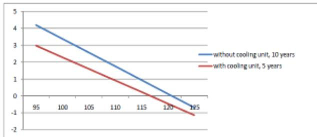
Fig. 2. CHP business model. PI as function of the fish cleaning waste price in two different cases: with a cooling unit and a 5 year lifespan for the CHP unit and without a cooling unit and a 10 year lifespan for the CHP unit. Economic duration of the project: 10 years.
