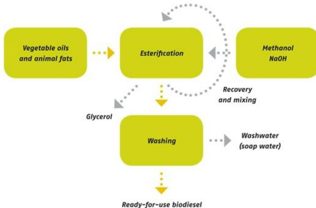
**Figure 5. Preseco biodiesel production process using transesterification (Preseco 2009).**
