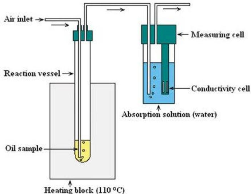
**Figure 6. Schematic of Rancimat test setup (Steinbach 2007).**
