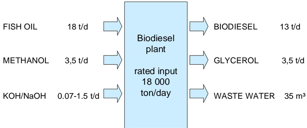
**Figure 3. Biodiesel production process.**
